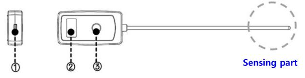
① USB port : Connect the sensor to a PC and use it for experiments or charging.
