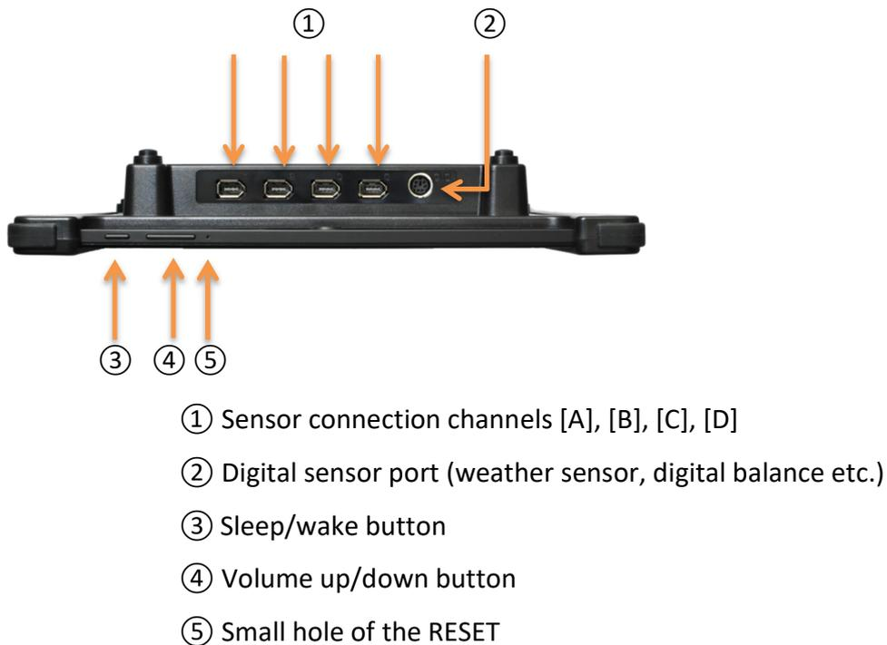
You can use the power switch (sleep/wake button) on the top side to power on MAX-A2, boot Android OS and start **Science#** application from display.
